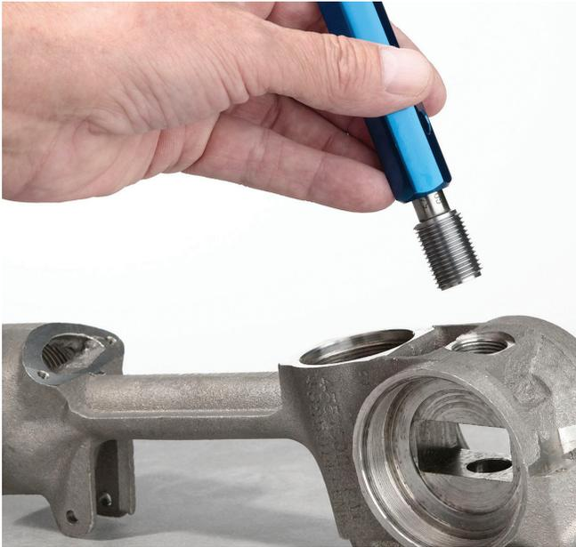
**CLASSES OF THREADS AND TAP SIZE:** There is a direct relationship between the size of a tap and the size of the thread that it cuts. Size refers to pitch diameter and its relationship to the class of fit required. If two threaded parts are assembled, the looseness or tightness of the fit is determined by contact on the flanks of the threads only. This contact is controlled by the pitch diameters of each part.
